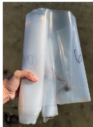
Pre-labeled, heat-sealed slots make it easier to sample and process, both in the field and in the lab.
